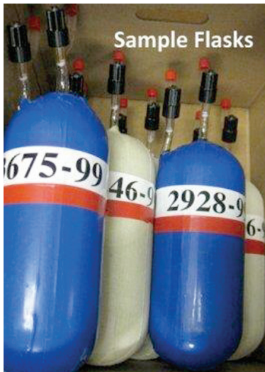
Fig. 7.30 Glass flasks used for collecting air samples. Air samples are taken in pairs as a quality assurance step (source: https://www.esrl.noaa.gov/gmd/ccgg/behind_the_scenes/surface.html )
