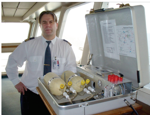
Fig. 7.32 Portable sampling unit installed on the bridge of STENA BALTICA operating in the Baltic Sea region; in the picture - Włodzimierz Jarzyński - one of the mates on the STENA BALTICA involved in air sampling supervised by MIR→NMFRI (1992-2011) (source: picture made available by W. Jarzyński)
