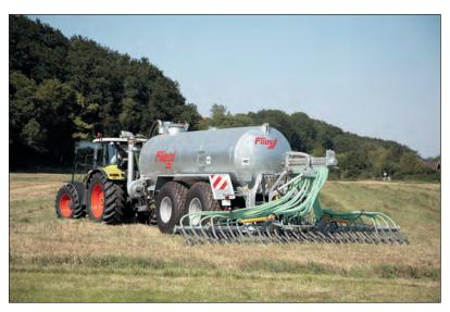
Photo 5.6 The modern slurry tank with applicator to shallow injection of liquid manure (photo by P. Nawalany)
